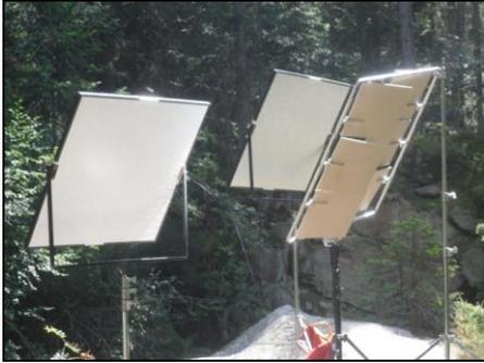
*Reflector panels used to strengthen sunlight*
